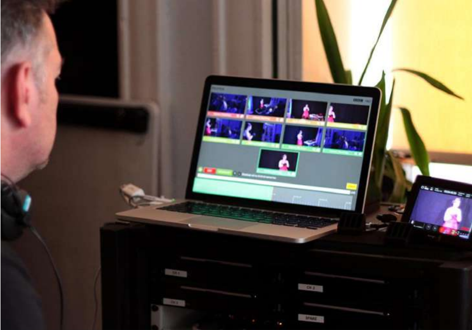
Fig 1: The SOMA tool allows a single operator to control several cameras and perform vision mixing using commodity hardware.
